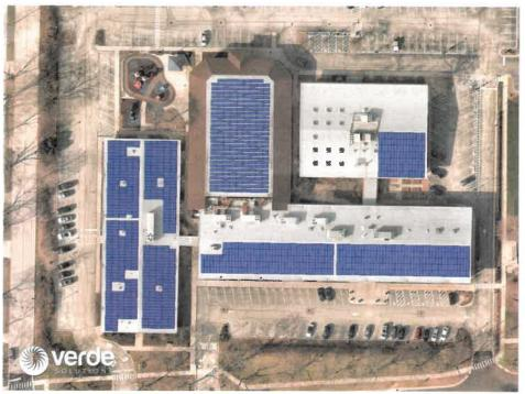
Figure 2: Proposed Solar System Design
